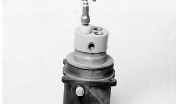
Center Joint Air Test
