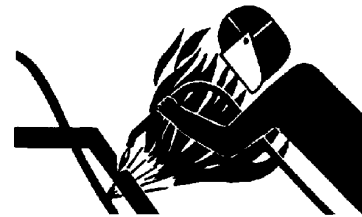
Heating Near Pressurized Fluid Lines
