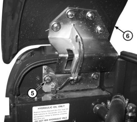
Upper Maintenance Access Door
